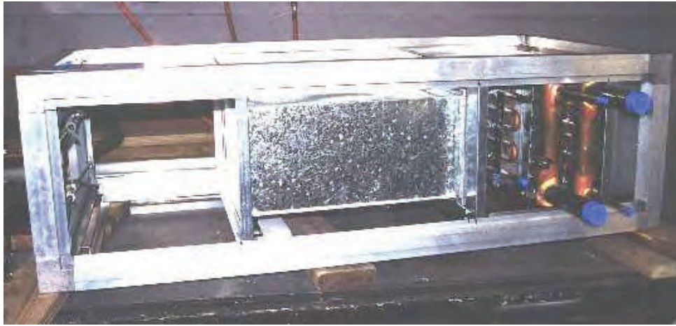
Figure 3.1. Side View before Panel is Installed showing frame, fan section, coils, and filter bolt assembly.
