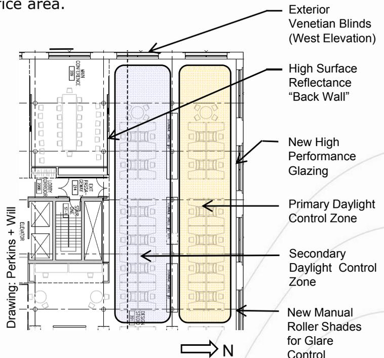
Photo control zones are grouped relative to daylight availability. Electric light sources are automatically dimmed when daylight is present. Manual over-rides give users the ability to manually turn electric lights off when not needed. Photocells are located in-plane with electric light fixtures in each zone.
