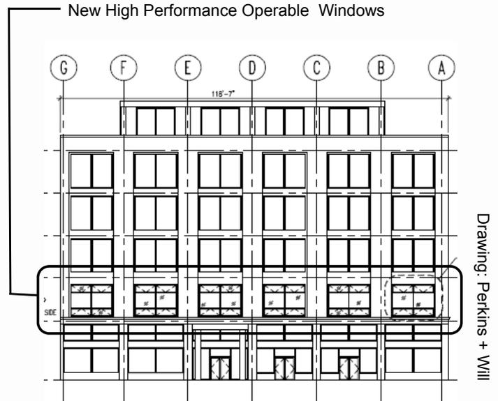
As part of their tenant improvement, Perkins+Will provided new operable high-performance windows. This enabled high visible light transmission with better solar control and a lower U-Value. This combination of increased thermal performance and light admittance saves energy on heating, cooling, and lighting. The operable sashes enable cross ventilation and passive cooling.
