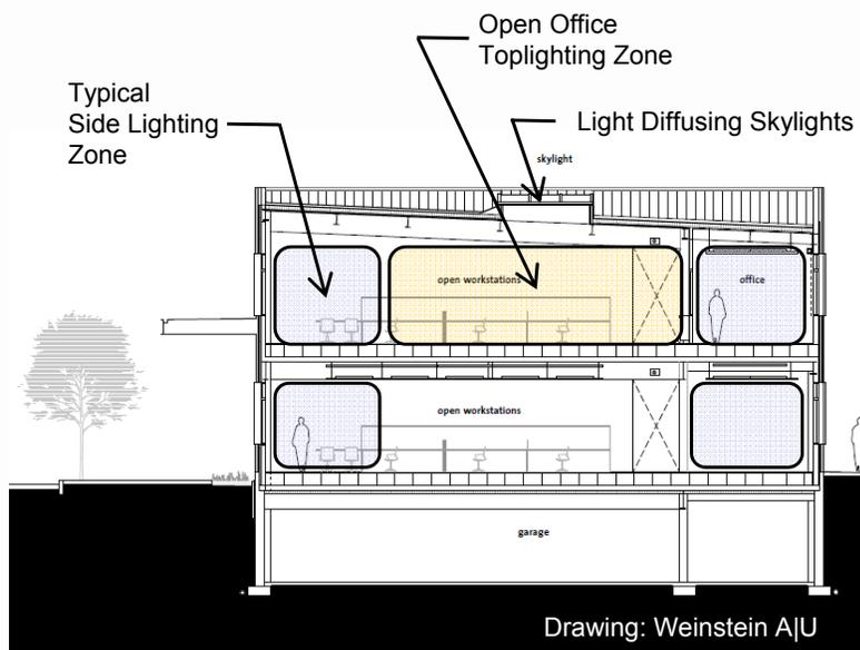
Sky-lit open office area with all general lighting controlled off via photo-cell. High efficiency accent and aisle way lighting provides sparkle and focal points. Re-lites through provide offices enables views to the exterior.
